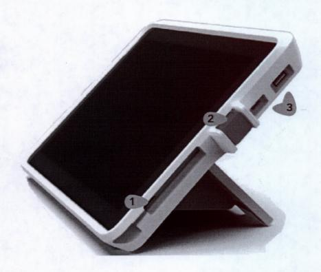
The ExpressPoll Flip Stand is a compact hardware option that integrates all necessary peripheral devices into the stand. This enclosure securely houses the tablet and includes two external USB hubs and utilizes the tablet's rear-facing camera to read barcodes. The ExpressPoll Flip Stand also features a unique kickstand with "barn doors" which allow the tablet to be flipped to capture voter signatures and other voter interactions.
